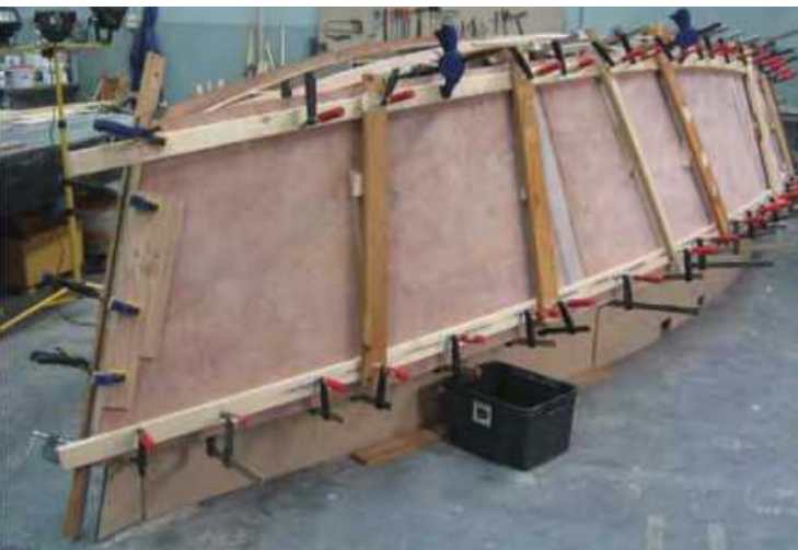
Figure 3 : Clamps and straps in place: only three screws.
