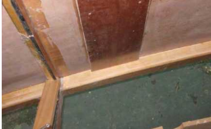
Figure 2 : Butt strap resting on sheer clamp.
