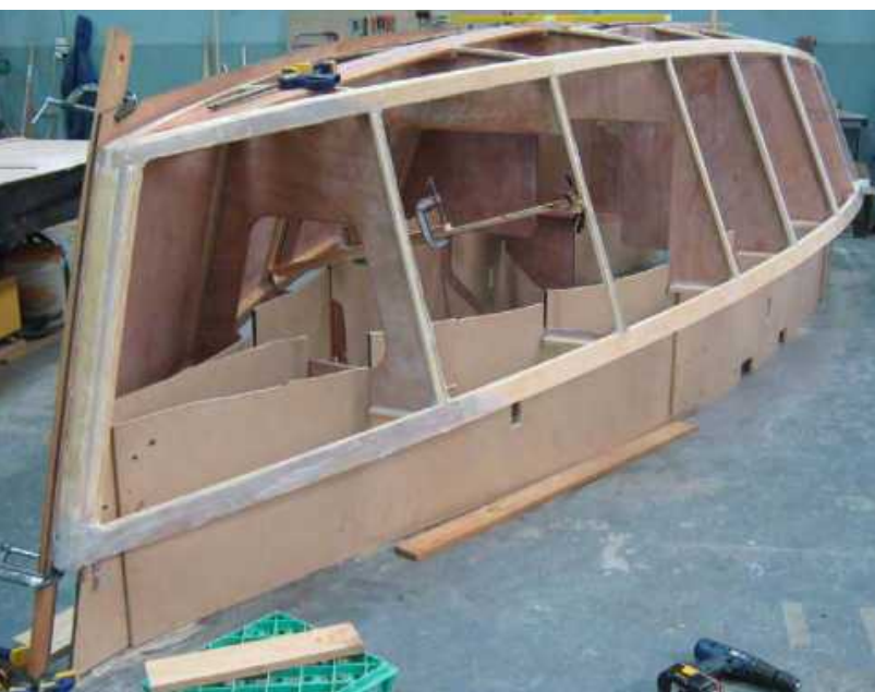
Figure 1 : Building jig trimmed for easy access. Note cross-bracing on bulkhead B.
