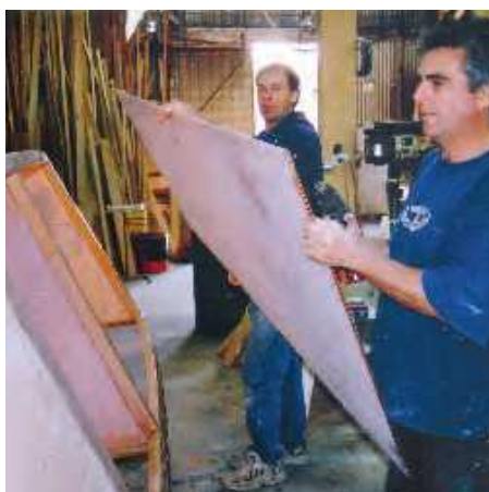
Stages of construction: above , no roof – the moulds are still inside the hull; right , adding a pre-cut panel, and, below , on goes the pre-fabricated roof
