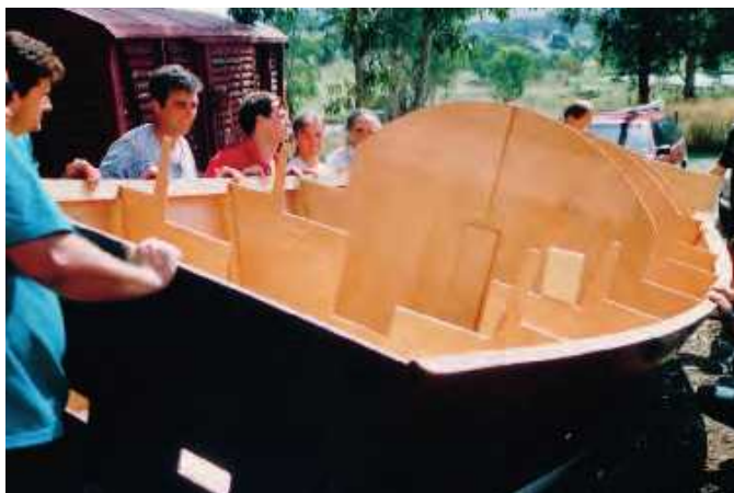
Stages of construction: above , no roof – the moulds are still inside the hull; right , adding a pre-cut panel, and, below , on goes the pre-fabricated roof
